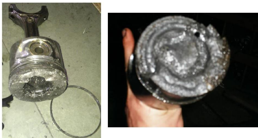
Figure 2: Severe overheat failure of engine piston [4].
