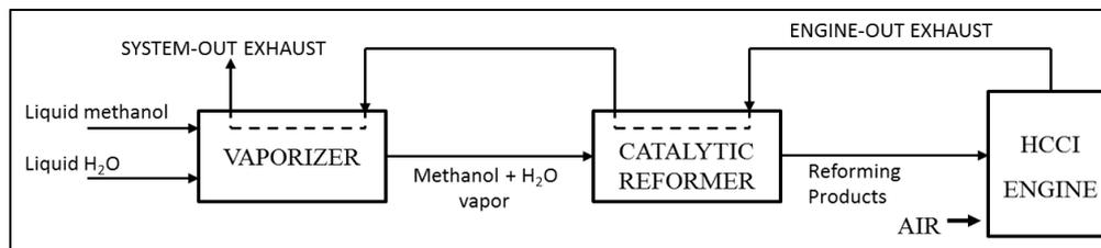
Figure 8. HCCI engine with thermo-chemical recuperation of the exhaust gas energy
