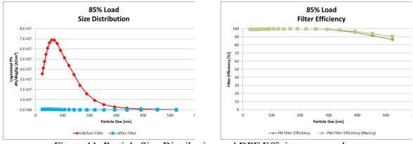
Figure 11: Particle Size Distribution and DPF Efficiency example
