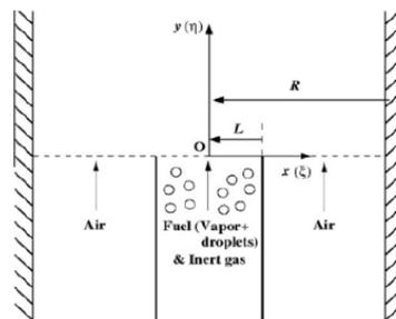
Fig. 1. Configuration for formation of Burke-Schumann spray diffusion flame.
