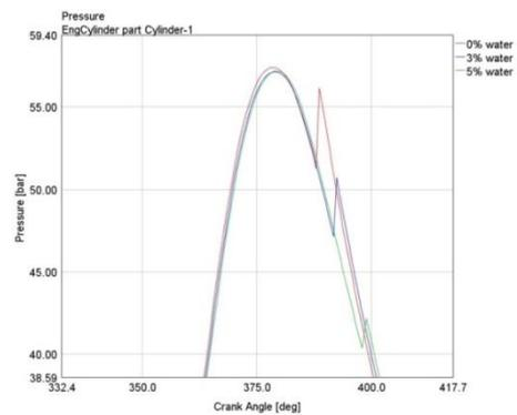
Figure 5. Peak pressures with 0, 3 and 5% mass water injection.
