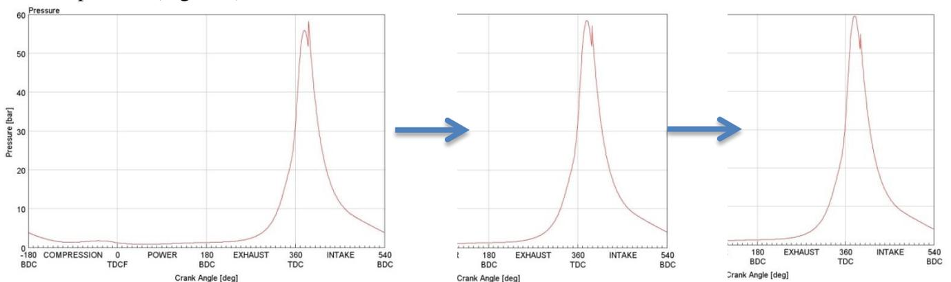
Figure 2. Indicator diagrams of Cylinder 1 at 330, 310 and 300 deg. Kelvin
