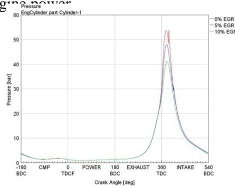
Figure 3. Indicator diagrams of Cylinder 1 with EGR
