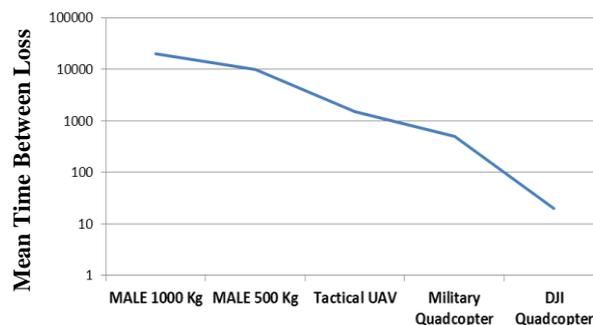
Figure 1. Mean time between loss and Platform size
