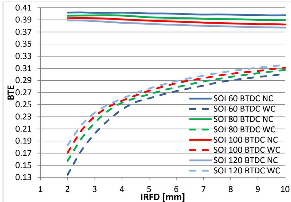
Figure 2. Dependence of BTE on IRFD and SOI values. SRM mixture (75% H<sub>2</sub>, 25% CO<sub>2</sub>), P<sub>b</sub> =75 kW, n=4,000 rpm, injection temperature =350K, reforming pressure 1 bar NC-compression power consumption not accounted for, WC-compression power accounted for (Poran, 2015).
