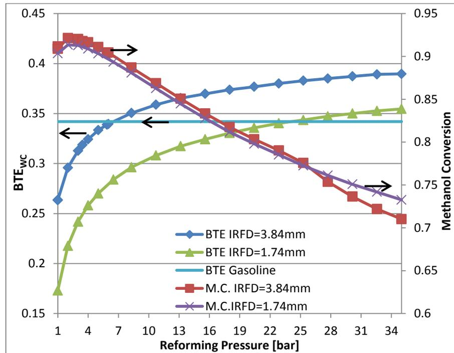
Figure 3. Dependence of BTE and methanol conversion (M.C.) on reforming pressure.  $P_b=75$  kW,  $n=4,000$  rpm, WOT,  $\lambda=1.2$ , reformer heat transfer area= $1.78$  m<sup>2</sup> (Poran, 2015).
