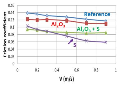
Figure 1. Comparison of friction between different treatments and a reference surface
