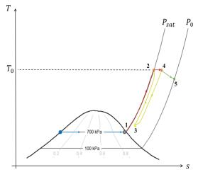
Figure 2. T-s diagram of the proposed cycle
