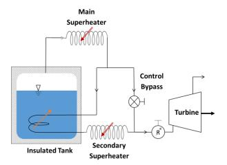
Figure 1. Schematic of the PCM engine concept
