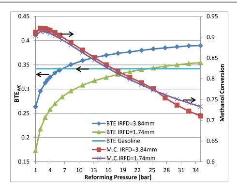
Figure 3. Dependence of BTE and methanol conversion (M.C.) on reforming pressure.  $P_b=75 \text{ kW}$ , n=4,000 rpm, WOT,  $\lambda=1.2$ , reformer heat transfer area=1.78 m<sup>2</sup> (Poran, 2015).
