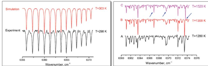
Fig.2 Left panel: FLICAS spectrum of CO<sub>2</sub> at room temperature along with simulation; Right panel: FLICAS spectrum of water vapors (A) at 1280 K along with simulation using original HITRAN database (C) and the modified one (B) (shifted lines shown with arrows), indicating the deficiencies of the spectral database.
