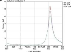
Figure 3. Indicator diagrams of Cylinder 1 with EGR
