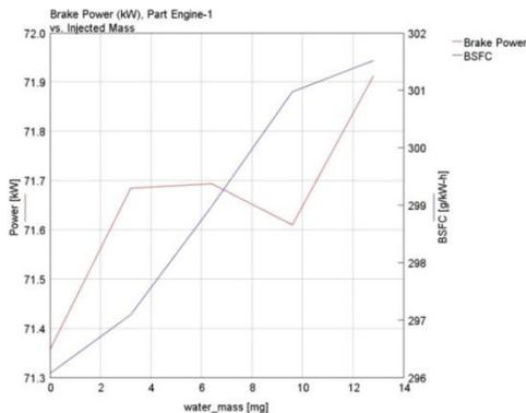
Figure 4. BSFC and brake power with water injection.
