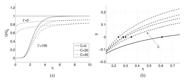
Figure 1: (a) Droplet mass fraction distribution as a function of the similarity coordinate for different values of the evaporation coefficient, C, and the vortex strength,  $\Gamma$ . (b) Schvab Zeldovich parameter shows the flame location where  $\beta = 0$ .
