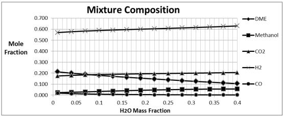
Figure 9. Reformate composition vs water mass fraction in the primary fuel
