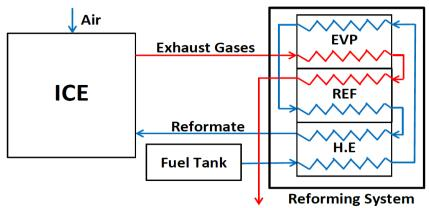
Figure 7. Flow chart of the ICE-SRM system. EVP-evaporator & super-heater, H.E-heat exchanger, REF-reformer
