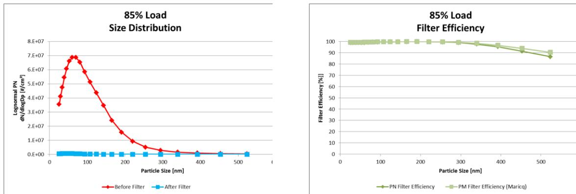
Figure 11: Particle Size Distribution and DPF Efficiency example
