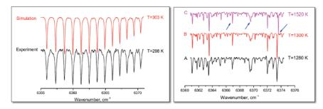
Fig.2 Left panel: FLICAS spectrum of  $CO_2$  at room temperature along with simulation; Right panel: FLICAS spectrum of water vapors (A) at 1280 K along with simulation using original HITEMP database (C) and the modified one (B) (shifted lines shown with arrows), indicating the deficiencies of the spectral database.
