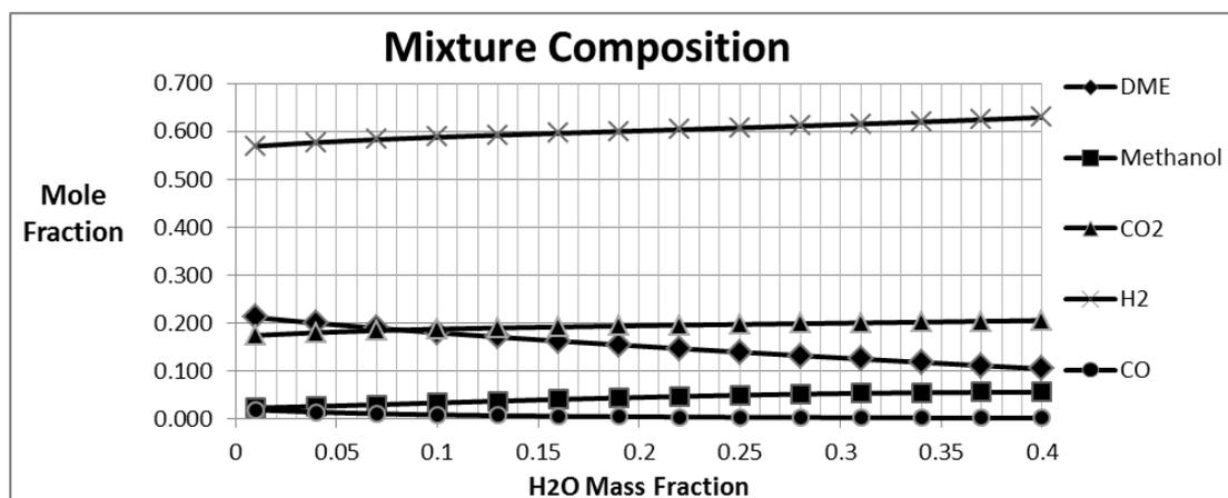
Figure 9. Reformat composition vs water mass fraction in the primary fuel
