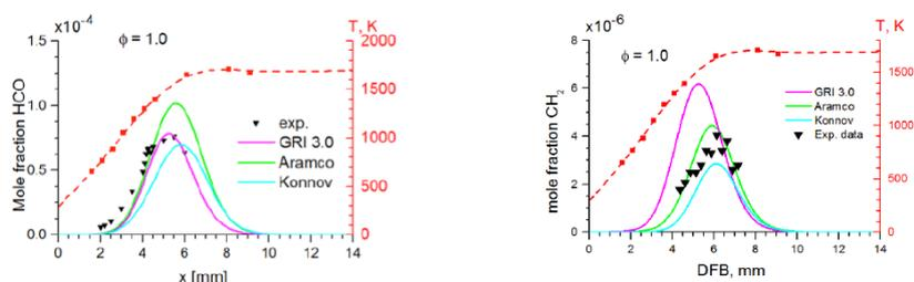
Fig.1 Experimental HCO(left) and CH<sub>2</sub>(right) profiles (filled triangles) and those calculated using the GRI mechanism (solid magenta line), Aramco mechanism (solid green line) and Konnov mechanism(solid blue line). Equivalence ratio is  $\phi = 1.0$ . Red diamond: temperatures measured by LIF.
