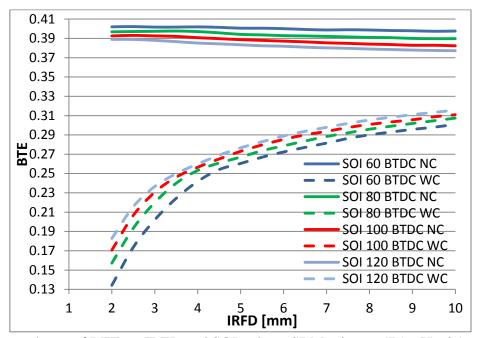
Figure 2. Dependence of BTE on IRFD and SOI values. SRM mixture (75%  $H_2$ , 25%  $CO_2$ ), P<sub>b</sub> =75 kW, n=4,000 rpm, injection temperature =350K, reforming pressure 1 bar NCcompression power consumption not accounted for, WC-compression power accounted for (Poran, 2015).
