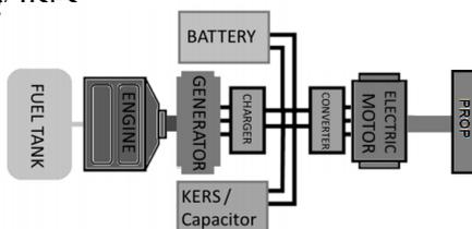
**Figure 12. Schematic Series Hybrid Propulsion System consumption**
